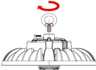
1. Install the hook into the fixture
