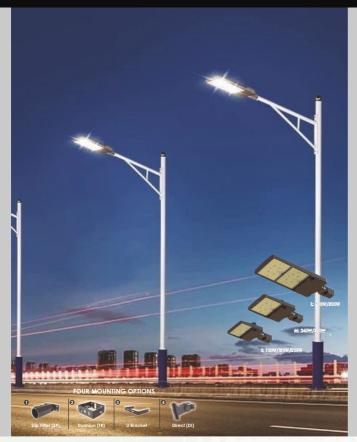
SIZE S, M, L WATT S:100/150/200 M:240/300L:400/500 CCT 3000K / 4000K / 5000K OR 4000K / 5000K / 5700K DIMMABLE 0-10V CRI LUMINOUS EFFICACY (Lm/W) UPTO 160 Lm/W **INPUT VOLTAGE** 120-277V or AC 120-480V or AC 200-480V IP RATING IP 65 Rated **OPERATING TEMPERATURE** -40°C ~ +45°C **POWER FACTOR** > 0.90 TOTAL HARMONIC DISTORATION (THD ≤ 20% LIFE SPAN 50.000+ Hrs
